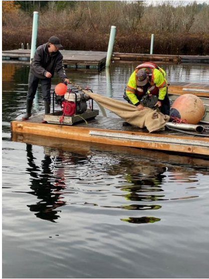
Photo 1. Venturi Pumping System with burlap collection bag
