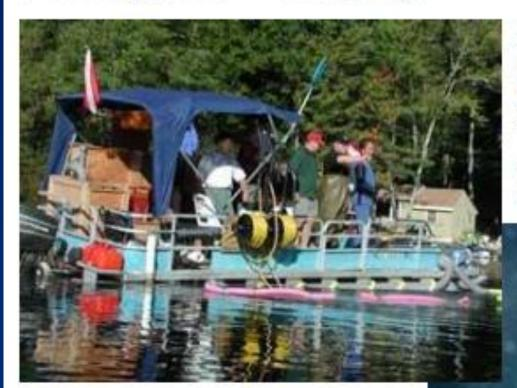
Suction pumps are used to transport plant material and mud into settling ponds on shore.
